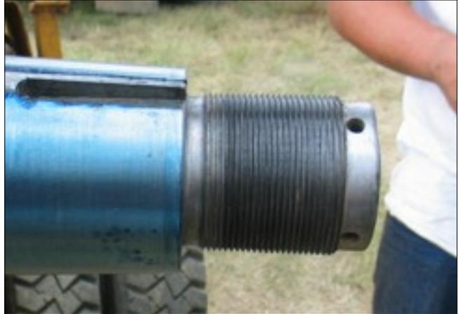
**Step 10:** Insert cotter pin in slot in castle nut, passing through hole in crank pin shaft. Bend ends of the cotter pin to insure that nut does not come loose.
