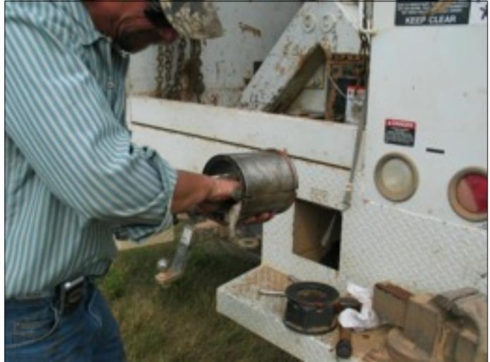
**Step 2:** Clean crank pin sleeve free of dirt and debris, inside and out using kerosene or 180# cleaner, followed up with 400# emery cloth. Never apply a thin film of lubricant to sleeve.
