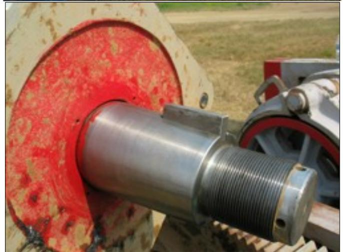
**Step 5:** With key installed on crank pin shaft, align crank pin assembly evenly with sleeve in bore. Align key with keyway in sleeve.
