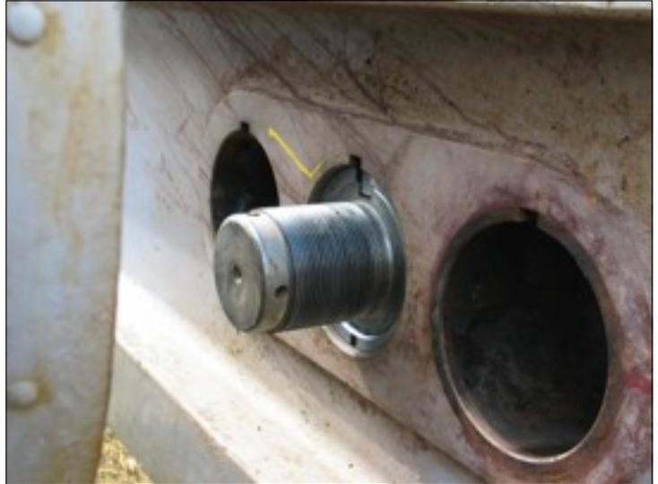
**Step 7:** Place crank pin washer over threaded end of crank pin shaft against crank arm.
