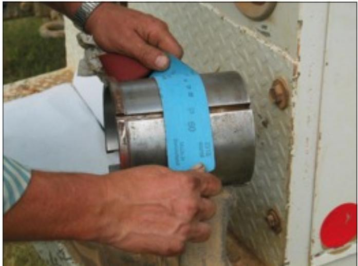
**Step 3:** Insert sleeve into crank bore while aligning keyway cut-out in sleeve with keyway in crank arm. Sleeve should slide freely into crank bore. It should not be necessary to beat the sleeve into the bore with a hammer. If sleeve meets resistance, check for burrs or high spots on sleeve and bore and file them if necessary
