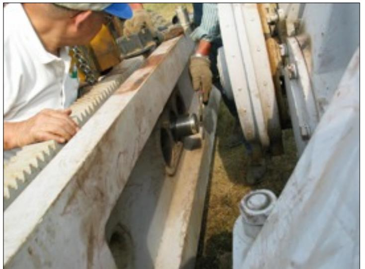
**Step 8:** Install crank pin castle nut on threaded crank pin shaft. Hand-tighten nut securely against washer.
