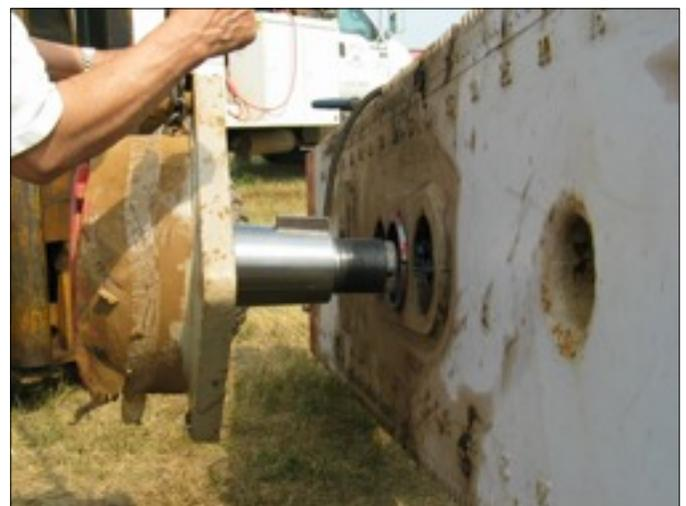
**Step 6:** Push crank pin assembly into sleeve in crank bore until crank pin assembly will not move any further. Key should be inserted with crank pin shaft,
